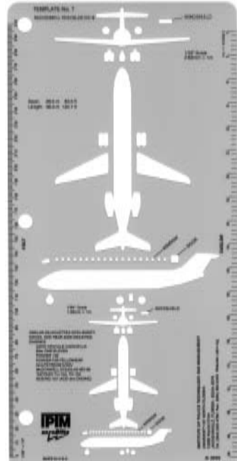
Template No. 7 (DC-9) is also suitable for non-scale diagrams of similar aircraft such as the Aerospatiale Caravelle, BAe One-Eleven, Fokker 1000, McDonnell Douglas MD-80, Tupolev TU-154 and Boeing 727 (with the addition of the third engine).
